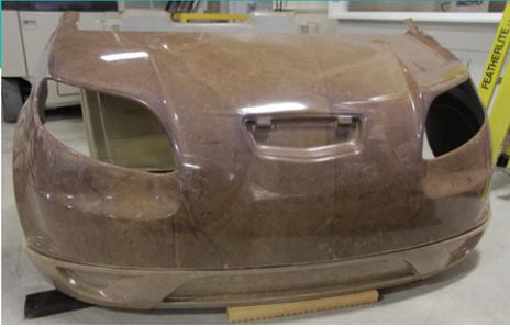
Fabricated prototype of a vehicle hood.
