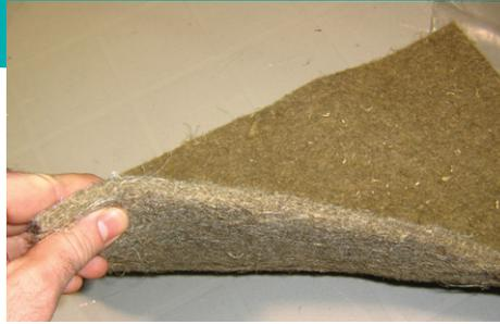
Biofibers used to reinforce composite structure.
